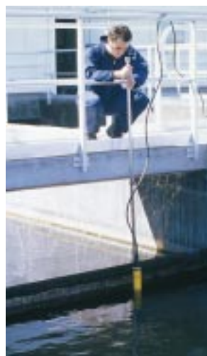
Measurement of liquid velocities using an acoustic doppler velocity probe (ADV) connected to a PC.
