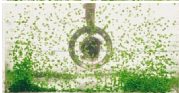
The importance of good mixer positioning: test results with the mixer in a good position (top), and in a less satisfactory position (bottom).
