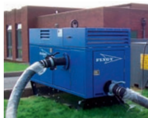
DWV Sewage by-pass pump
